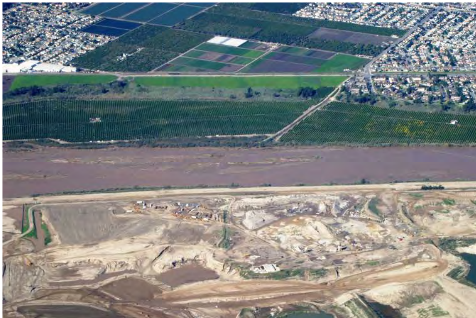
Figure 5-11. View across the Santa Clara River in Reach 2 (near Saticoy) on the lower Santa Clara River showing the 1961 Army Corps of Engineers levee (left bank) during the recession of the 2005 flood. Active floodplain aggregate mining in the foreground. (Photo courtesy of the California State Coastal Conservancy)
