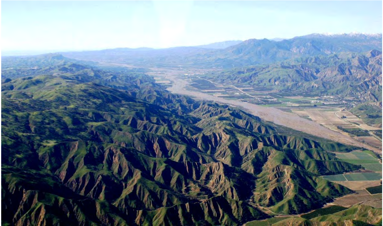
Figure 4-2. January 2005 view of the Santa Susana Mountains (left and foreground) and Santa Clara River near the confluence of Piru Creek (downstream, westward view). Slopes in the watershed exhibit numerous landslide scars, including many that span entire hillslope lengths, from ridgetops to channel bottoms. Note snow capped peaks at upper right. (Photo courtesy of the California Coastal Conservancy)
